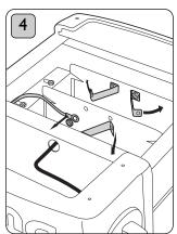
Bend brass links and wires away from the element.
